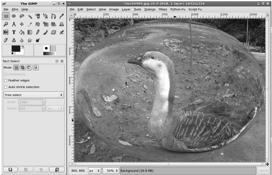
Figure 20-8. The Glass Effects ▶ Apply Lens filter can be used to imitate a fish-eye lens.
