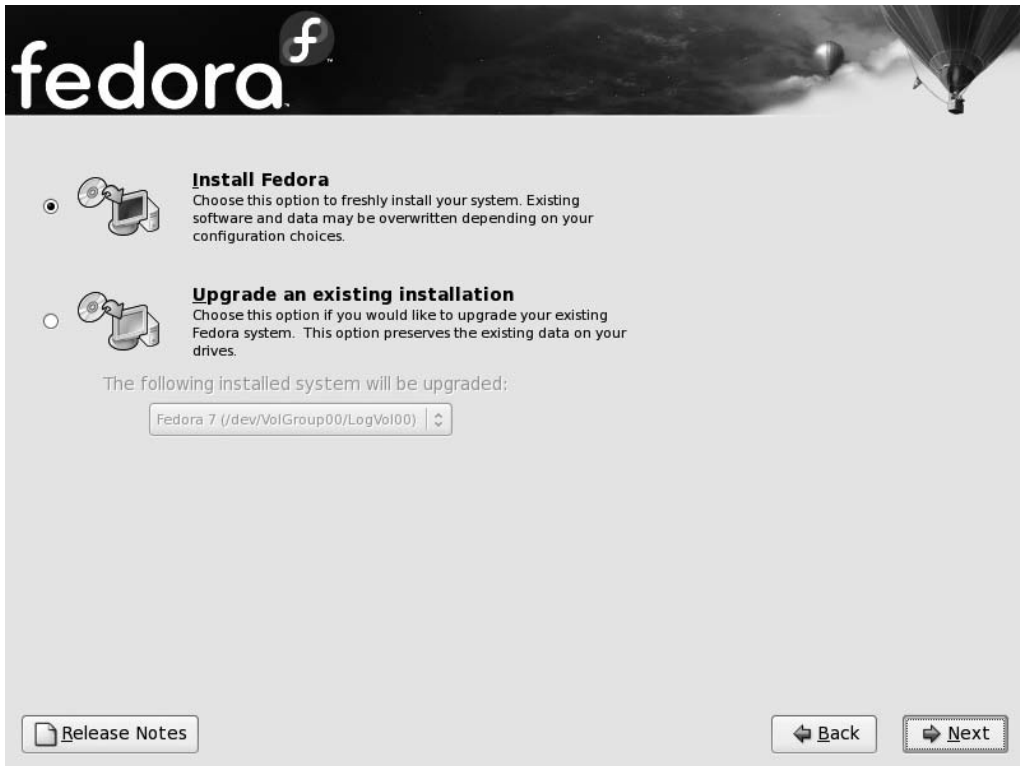
Figure 5-4. Fedora will automatically discover any existing installations and allow you to upgrade or do a fresh install.
