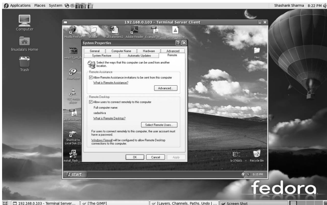
Figure 33-4. You can access remote Windows XP Professional machines using RDP and the Terminal Server Client program.
