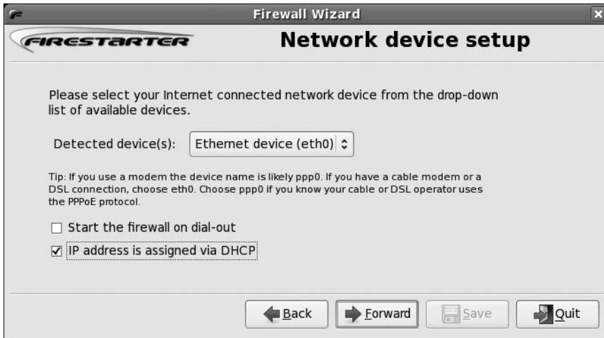
Figure 9-4. Firestarter includes a wizard to walk you through the basics of firewall configuration.
