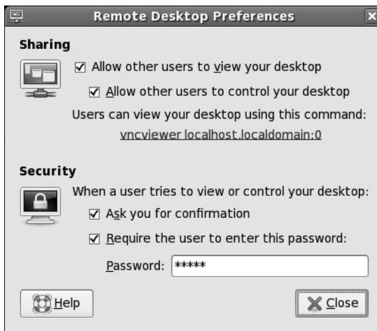
Figure 33-2. Fedora's Remote Desktop feature lets you share your desktop, but isn't as secure as making an X server connection with ssh .
