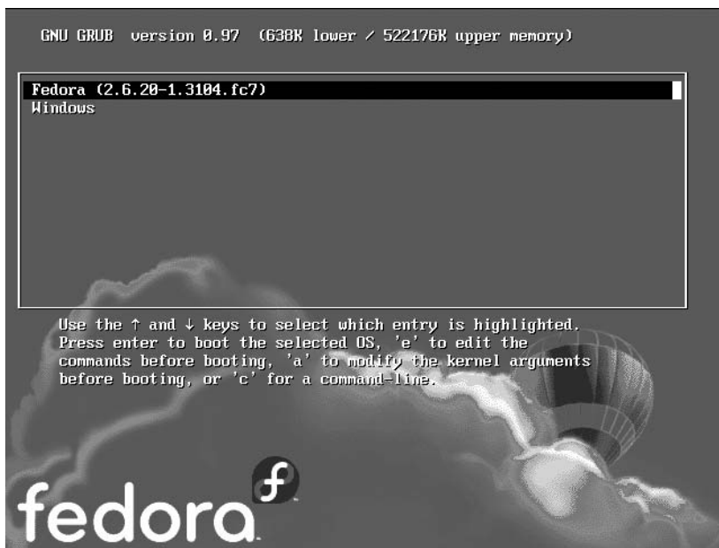
Figure 7-1. The default choice is fine on the boot menu, so press Enter to start Fedora.
