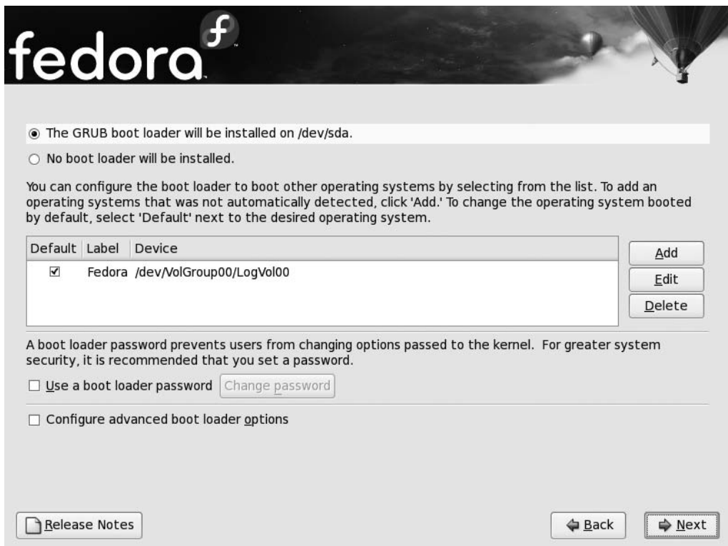
Figure 5-8. The GRUB boot loader is the menu that appears when you boot, allowing you to choose between Fedora and Windows.
